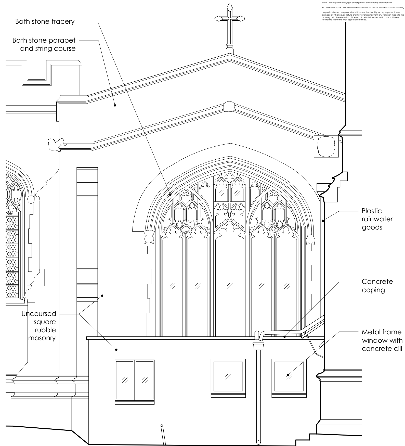
West Elevation | As Existing
